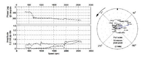
**Fig. 4.** Bode and polar plots following the axial redistribution of weights based on influence coefficients obtained through the previous two trial runs.
