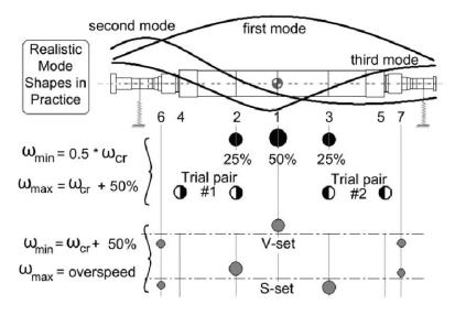
Fig. 1. Identification of balancing correction planes and possible weight distributions
