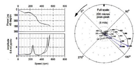
**Fig. 2.** Bode and Polar plots of the first run showing high amplitudes approaching the first critical speed, used to determine the direction of the static unbalance vector
