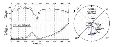
Fig. 3. Bode and Polar plot following the initial first critical correction in 3 planes.
