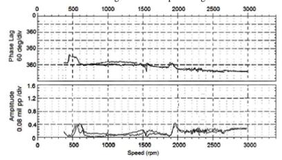
Fig. 5. Final Bode plot of the fully balanced generator rotor
